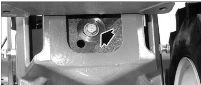
Figure 5-1: Check bolt on transmission pulley.
